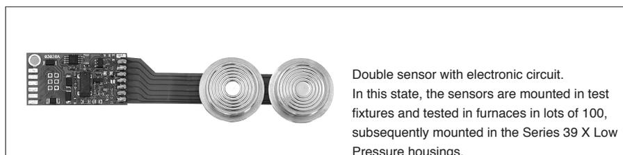
Double sensor with electronic circuit.
